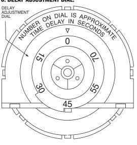
NOTE: RETARD TIME MAY EXCEED 90 SECONDS ADJUST AND VERIFY THAT TIME DOES NOT EXCEED 90 SECONDS NUMBER ON DIAL IS APPROXIMATE TIME DELAY IN SECONDS WITH AN ACCURACY OF +/- 50%
