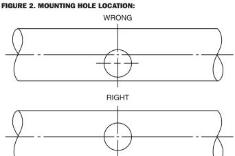
REMOVE BURRS FROM EDGE OF HOLE. CLEAN OUT SCALE AND FOREIGN MATTER FROM INSIDE WALL OF PIPE.
